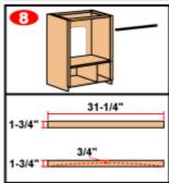
Cut a moveable shelf from your plywood, sand the exposed edge and glue it into position. Then cut the shelf door from edge-glued oak stock.
