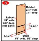
4. Cut a dado on each of the fixed shelves, as shown from the door end. Then, on the side panel that will have the door, drill a pair of holes from the front and rear edges, for the shelf support pins. On the cabinet side, they should be above the fixed shelf. Drill corresponding holes on the partition from the lower edge.
