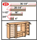
24. Now cut the trim pieces from your solid oak stock. Cut them a little long, and then round over the long edges. Round over one end of each side trim, then trim them to fit, and miter the inner ends. Also miter the matching end of the shortest trim piece, leaving the remaining end square.
