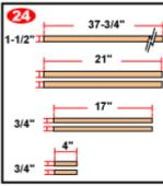
25. Cut the center skirt and two side skirts from your solid oak stock and round over all four edges. Then sand all parts before installing.
