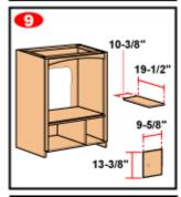
10. When building the audio rack module with adjustable shelves for holding tapes and CDs, start by constructing a lapframe similar to the one you made for the television unit. You'll again cut lapframe longs and shorts to size, and cut half laps like before. Use glue and clamps to connect sections.
