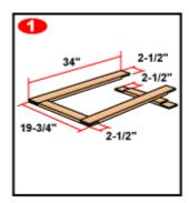
Cut to size the side panels, fixed shelves, the partition and the shelf edge strips. Glue the edge strips to the fixed shelves and the partition and allow the glue to dry before sanding the surfaces flush.
