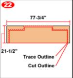
23. You'll now need to cut and mount filler strips from your spruce or pine stock. These will go under the top for the purpose of eliminating the gap that would otherwise occur behind the edge trim.
