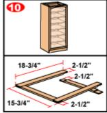
11. Cut to size the side panels and the two edge strips, the fixed shelf and its edge strip. Glue the edge strips to the sides and to the shelf, using clamps, tape or small finishing nails to hold them. When the glue is dry, sand the surfaces flush.
