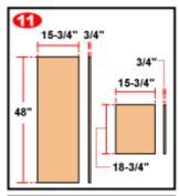
12. On a side panel, cut a rabbet along the inner rear edge, making sure the good side will face out. Cut a dado to length from the bottom edge, and then cut a rabbet along the top edge. Now cut corresponding dados and rabbets on the other panel, making sure the sides are mirror images and that the dados line up.
